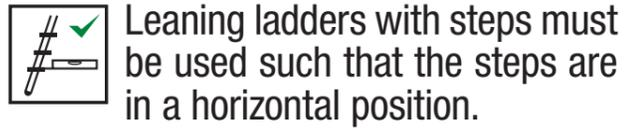
Leaning ladders with steps must be used such that the steps are in a horizontal position.
