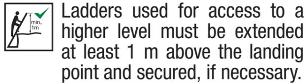
Ladders used for access to a higher level must be extended at least 1 m above the landing point and secured, if necessary.
