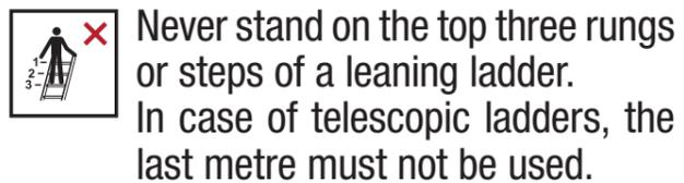
Never stand on the top three rungs or steps of a leaning ladder. In case of telescopic ladders, the last metre must not be used.
