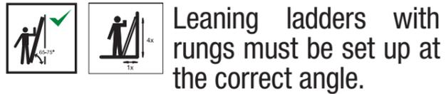
Leaning ladders with rungs must be set up at the correct angle.
