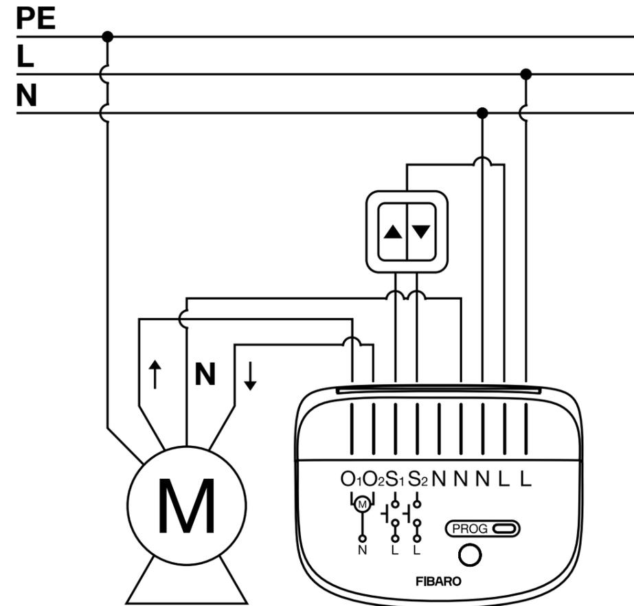
Wiring diagram - connection with AC motor
