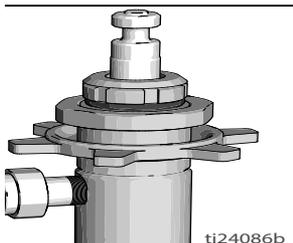
2. Move pump displacement rod up or down until it slides into the connecting rod when the pump is slid into the drive housing.
