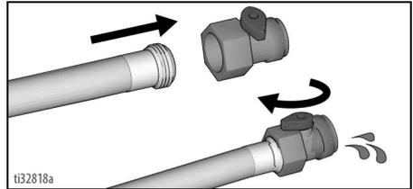
9. Unscrew inlet screen from Suction Tube. Place inlet screen in waste pail. Connect garden hose to Power Flush Valve on Suction Tube. Leave Drain Tube in waste pail.
