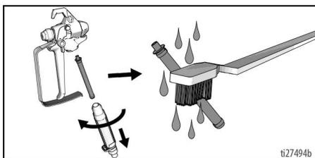
3. Clean gun filter with water or flushing fluid and a brush every time you flush the system. Replace gun filter if damaged.
