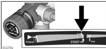
8. Turn ON/OFF switch to **ON** position.
