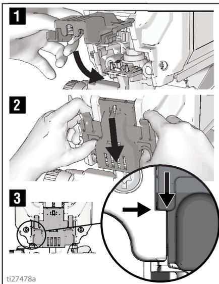
3. Install hose, suction tube, and drain tube.
