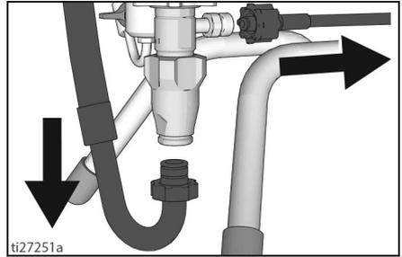
5. Slide pump out of the drive housing.
