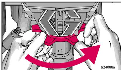
6. Use a hammer to turn pump retaining nut an additional 1/8 to 1/6th turn or 45° to 60°.
