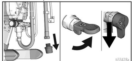
4. Place drain tube in waste pail. Turn pressure control to the **START** position.
