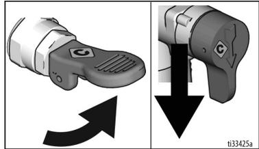
5. Hold the gun firmly to a pail. Point gun into pail. Disengage the trigger lock and trigger the gun to relieve pressure.
