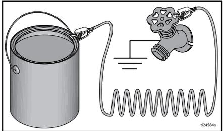
**To maintain ground continuity when sprayer is flushed or pressure is relieved:** hold metal part of gun firmly to the side of a grounded metal pail, then trigger the gun.
