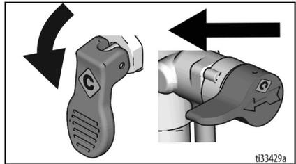
9. Turn ON/OFF switch to **OFF** position. Disconnect power (unplug power cord).
