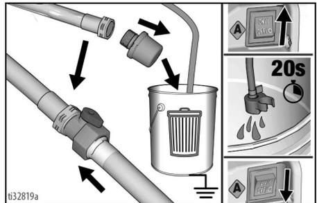
10. Turn ON/OFF switch to **ON** position.
