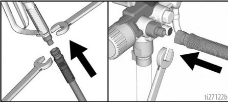
3. Assure Spray Tip is properly inserted into the Spray Tip Guard, and the Spray Tip Guard assembly is tightened securely to gun. See **Spray Tip Installation**, page 25.
