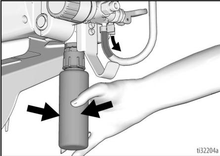
5. Remove tool. Replace and tighten child-proof cap for storage.
