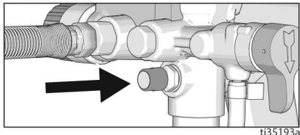
7. Align setting indicator with the **START** setting on the pressure control knob.
