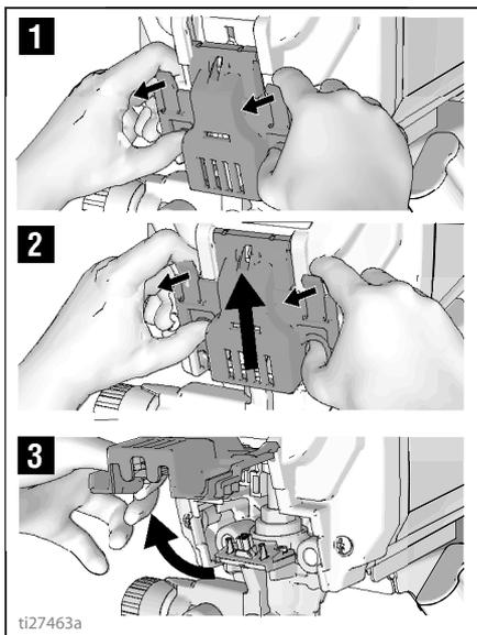
4. Slide pump assembly off the mounting pins.
