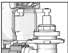
3. Slide pump all the way into drive housing.
