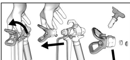
5. See **Spray Tip Installation**, page 25 to properly reinstall Spray Tip Guard assembly.
