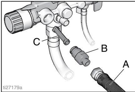
5. Check InstaClean Filter (C) for debris. If needed, clean filter with water or flushing fluid and a soft brush.
