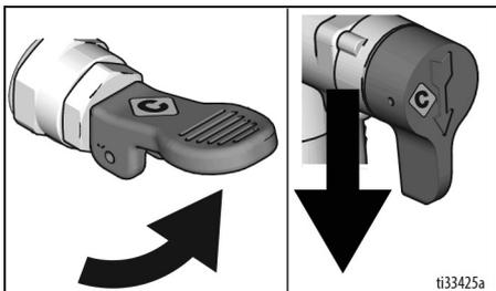
9. Turn ON/OFF switch to **ON** position.
