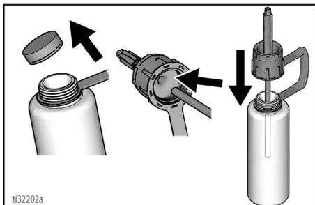
3. Remove sprayer Suction Tube. Insert tool into the inlet and push up firmly until it stops.
