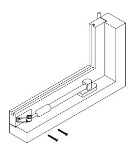
7. Set the friction one-off by using the turn button. You don't need to turn the restrictor while opening and closing the window.
