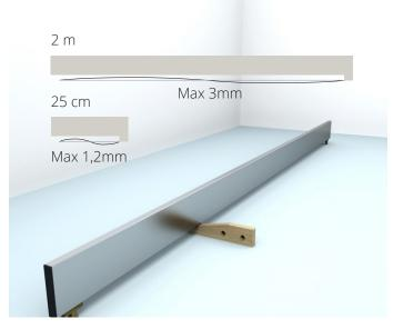
Without exception check that the subfloor is flat and level over measured lengths of 2m and 0.25m. If any unevenness exceeds +/- 3mm over 2m and +/- 1.2mm over 0.25m, the floor must be levelled prior to installation of the Aware floor. Kährs also accepts a measuring length of 1 m. The tolerance in this case is +/- 2mm.
