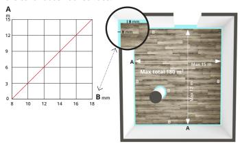
The size of the movement joint in mm is calculated using the formula: 2mm x 3-meter floor area. The size of the movement joint should never be less than 8mm. Remember to remove the spacers after installation is done and complete.
