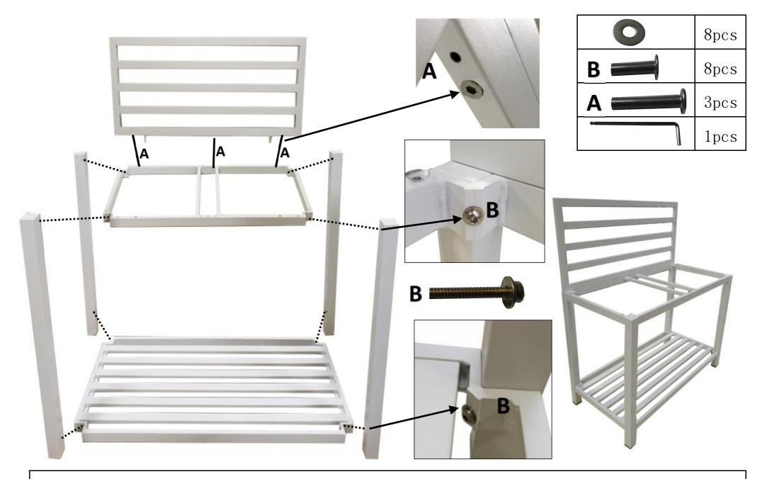
IMPORTANT: In order to make the whole product adjust to the best, please install all the screws on the product before fully tighten, and note to put the washer to the screw before putting the screw into the screw hole.
